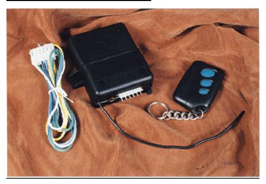
Location of the control module is the most important factor in range and reliability of your Code Encryptor. Select a location that is as centrally located as possible. Keep in mind that your customer will want to control the operation of his garage door from his driveway, and he will also expect the use of the remote for On/Off in the area of entry and exit.
